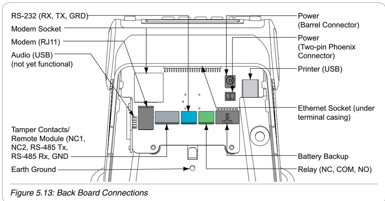
Figure 5.13: Back Board Connections
