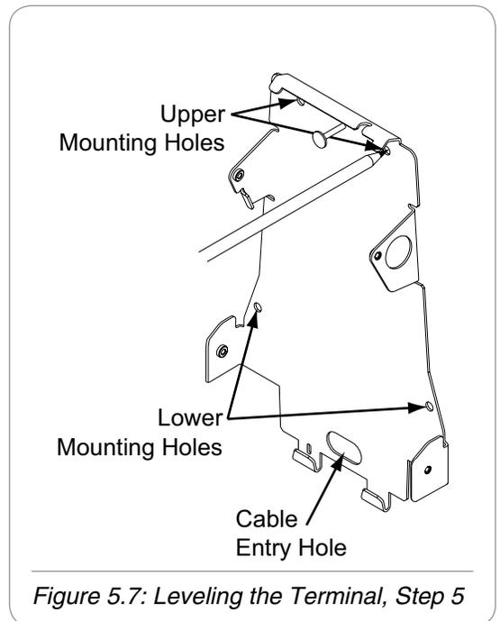
Figure 5.7: Leveling the Terminal, Step 5
