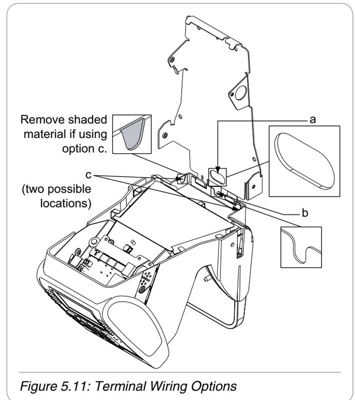
Figure 5.11: Terminal Wiring Options
