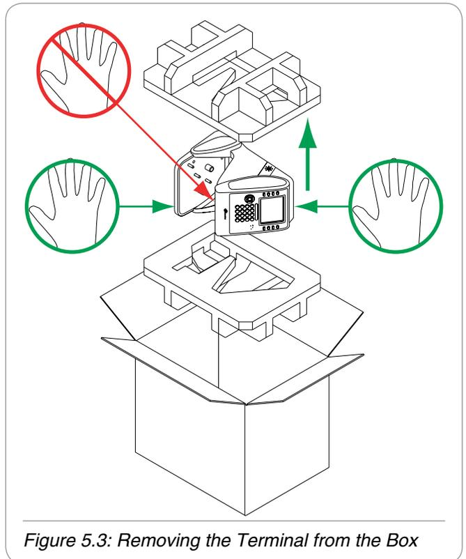
Figure 5.3: Removing the Terminal from the Box
