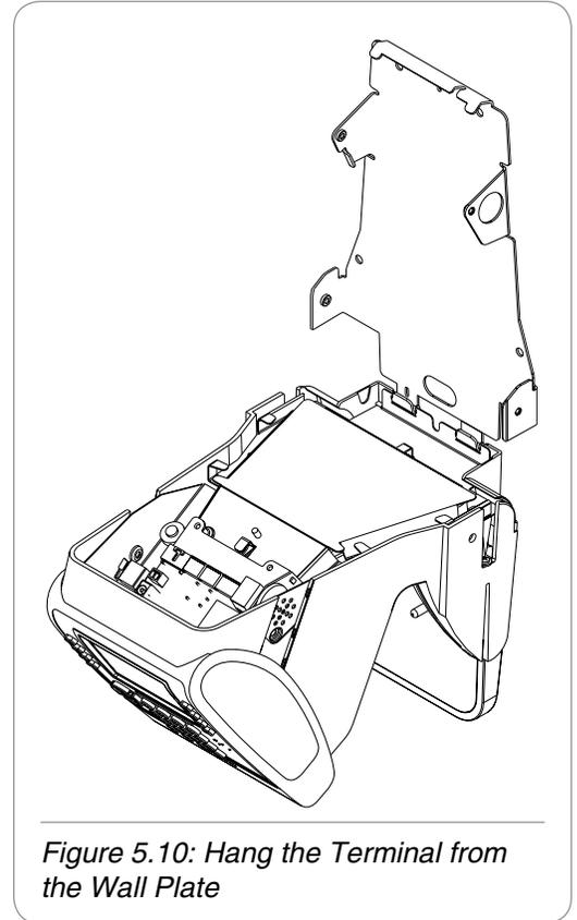
Figure 5.10: Hang the Terminal from the Wall Plate
